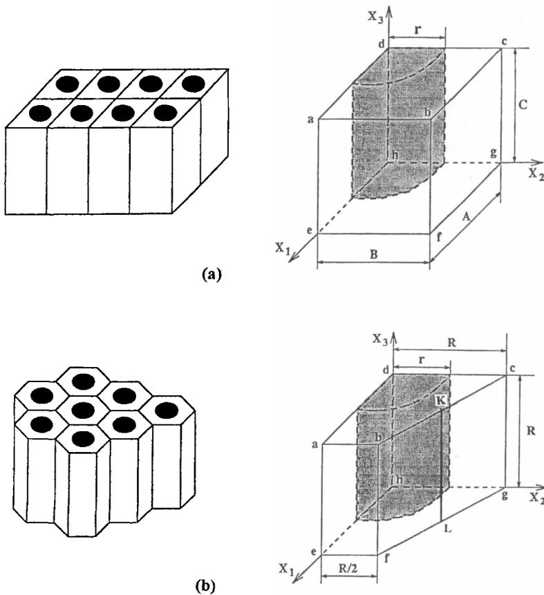
FIGURE 3 One-eighth of a representative volume element containing a cylindrical fiber: (a) the cubic or rectangular cell, (b) the hexagonal cell.
