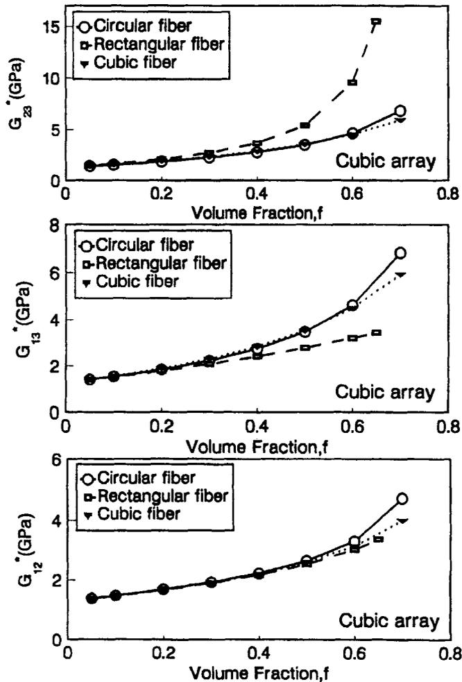
FIGURE 7 Effect of fiber shape for the cubic array on effective shear moduli.
