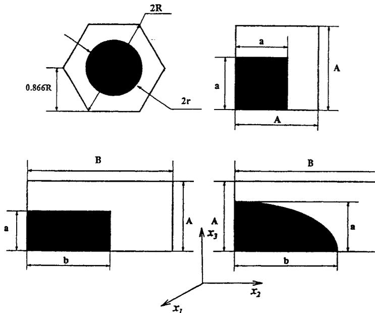
FIGURE 2 Schematic of four fiber shapes on the transverse plane.
