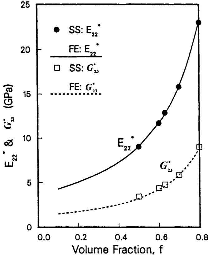
FIGURE 4 Comparison of  $E_{22}^*$  and  $G_{23}^*$  calculated from a series solution<sup>(11)</sup> and from the finite element method.
