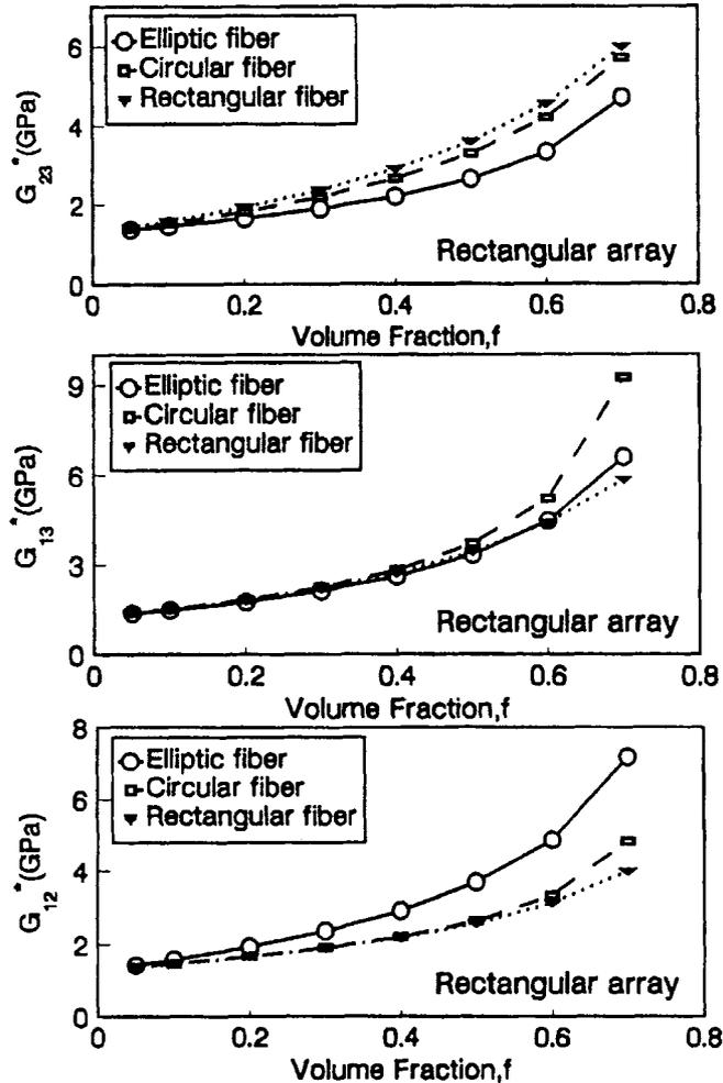
FIGURE 6 Effect of fiber shape for the rectangular array on effective shear moduli.
