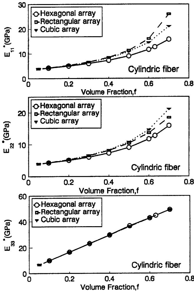
FIGURE 8 Effect of fiber packing array for the cylindrical fiber on effective Young's moduli.
