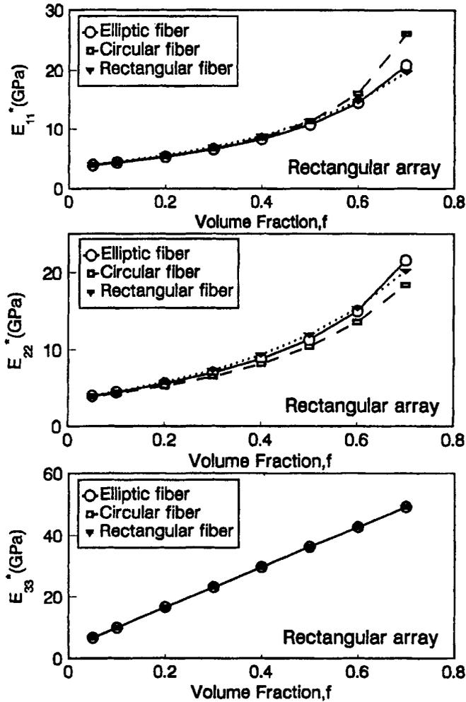
FIGURE 5 Effect of fiber shape for the rectangular array on effective Young's moduli.
